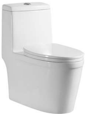
LX-2112 Rimless Siphonic One-piece Toilet Size:720x370x740mm Vitreous china S-trap,305/400 Rounghing-in
