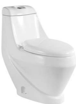
LX-2080 Washdown One-piece Toilet Size:750x385x735mm Vitreous china S-trap,250/300mm Rounghing-in P-trap,180mm Rounghing-in
