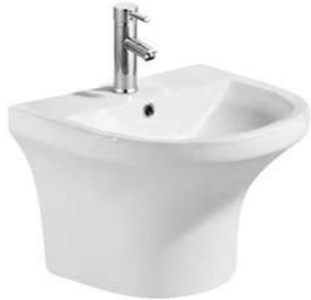
LX-3006 Wall-hung basin Size:440x500x350mm Vitreous china Fixing to wall with back
