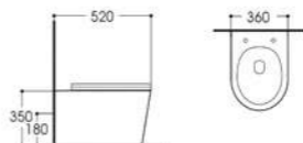
LX-1905 Rimless Washdown Wall-hung Toilet Size:520x360x350mm Vitreous china P-trap,180mm Rounghing-in
