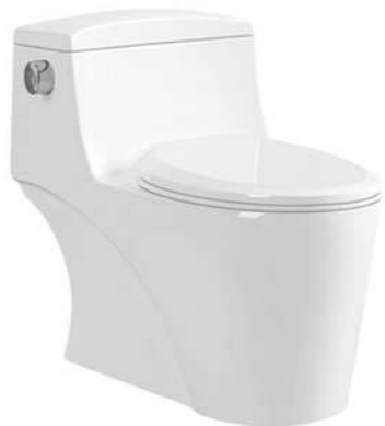
LX-2913 Siphonic One-piece Toilet Size:750x460x675mm Vitreous china S-trap,300/400mm Rounghing-in
