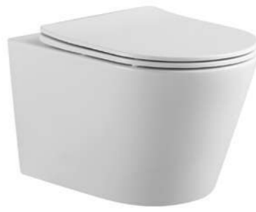
LX-1905 Rimless Washdown Wall-hung Toilet Size:520x360x350mm Vitreous china P-trap,180mm Rounghing-in
