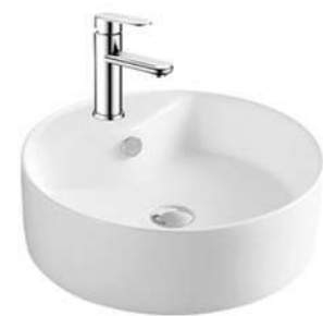
LX-5002A/5002B Art basin Size A:460x460x155mm Size B:410x410x145mm Above counter mounting
