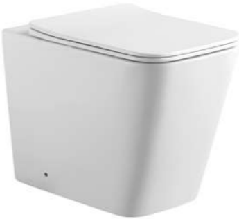
LX-1908 Floor standing toilet Size:540x345x410mm Vitreous china P-trap,180mm Rounghing-in
