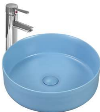
LX-7138 Art basin Size:355x355x115mm Vitreous china Above counter mounting
