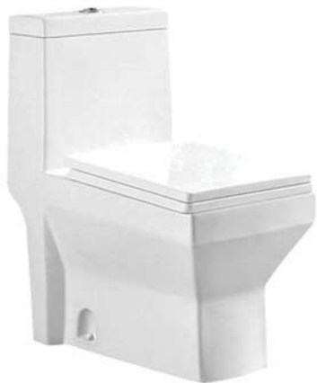
LX-2732 Washdown One-piece Toilet Size:690x370x780mm Vitreous china S-trap,250mm Rounghing-in P-trap,180mm Rounghing-in
