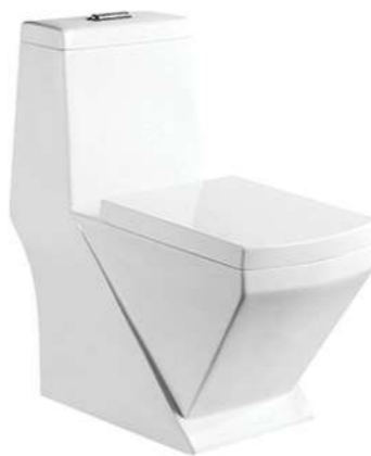
LX-2190 Rimless Siphonic One-piece Toilet Size:710x370x755mm Vitreous china S-trap,250/300mm Rounghing-in P-trap,180mm Rounghing-in
