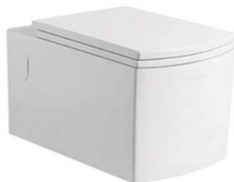
LX-1113 Washdown Wall-hung Toilet Size:600x385x350mm Vitreous china P-trap,180mm Rounghing-in
