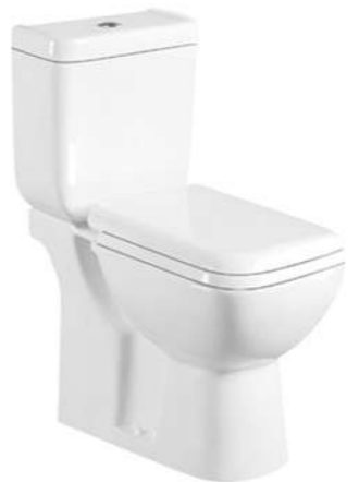
LX-2029 Wasdown Two-piece Toilet Size:650x370x795mm Vitreous china S-trap,250mm Rounghing-in P-trap,180mmRounghing-in
