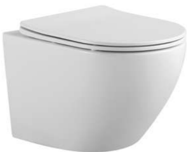
LX-1901 Rimless Washdown Wall-hung Toilet Size:520x355x340mm Vitreous china P-trap,180mm Rounghing-in
