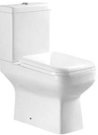
LX-2830 Wasdown Two-piece Toilet Size:650x365x790mm Vitreous china S-trap,250mm Rounghing-in P-trap,180mmRounghing-in
