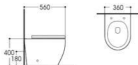
LX-1902 Floor standing toilet Size:560x360x400mm Vitreous china P-trap,180mm Rounghing-in
