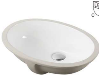
LX-6224 Under Counter Basin Outside Size:440x375x185mm 17 3/8"x14 3/4"x7 1/4" Inside Size:400x335mm 15 3/4"x13 1/5" Under counter mounting
