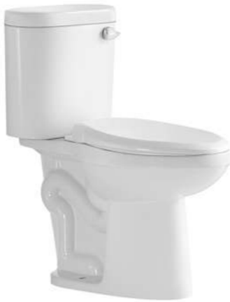
LX-2756D Siphonic Two-piece Toilet Size:705x400x810mm Vitreous china S-trap,300mm Rounghing-in
