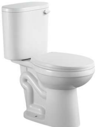
LX-2759D Siphonic Two-piece Toilet Size:680x400x795mm Vitreous china S-trap,300mm Rounghing-in
