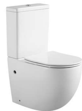
LX-2903 Washdown Two-piece Toilet Size:615x375x836mm Vitreous china S-trap,250 Rounghing-in P-trap,180mm Rounghing-in
