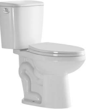
LX-2749B Siphonic Two-piece Toilet Size:725x390x815mm Vitreous china S-trap,300mm Rounghing-in
