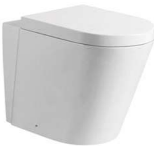
LX-1125 Washdown Close-couched Toilet Size:570x360x420mm Vitreous china P-trap,180mm Rounghing-in
