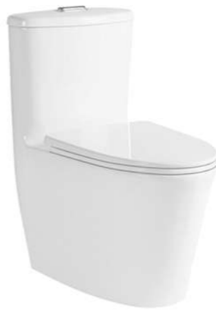
LX-2728 Rimless Siphonic One-piece Toilet Size:700x385x760mm Vitreous china S-trap,300/400 Rounghing-in
