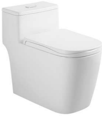
LX-2039 Rimless Siphonic One-piece Toilet Size:705x390x630mm Vitreous china S-trap,305/400mm Rounghing-in
