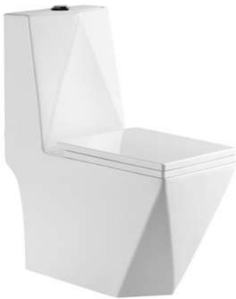
LX-2135 Siphonic/Washdown One-piece Toilet Size:680x380x830mm Vitreous china S-trap,250/300/400mm Rounghing-in P-trap,180mm Rounghing-in
