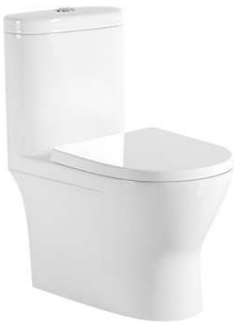
LX-2920 Siphonic One-piece Toilet Size:680x380x780mm Vitreous china S-trap,300/400 Rounghing-in
