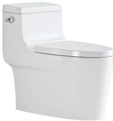
LX-2602 Rimless Siphonic One-piece Toilet Size:740x400x680mm Vitreous china S-trap,300/400mm Rounghing-in
