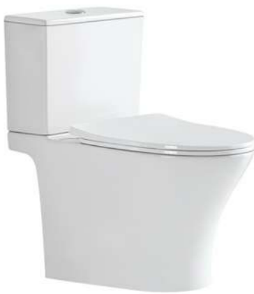
LX-2777 Wasdown Two-piece Toilet Size:720x370x740mm Vitreous china S-trap,250mm Rounghing-in P-trap,180mmRounghing-in
