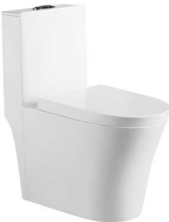
LX-2722 Rimless Siphonic One-piece Toilet Size:685x365x765mm Vitreous china S-trap,300/400mm Rounghing-in
