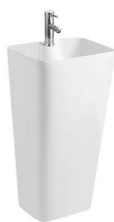
LX-8012 Pedestal Basin Size:460x430x830mm Vitreous china Fixing to wall with back
