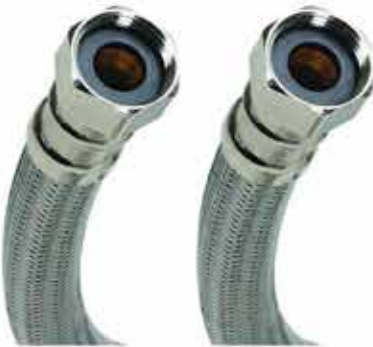
FMB1H24 3/4" FIP x 24" Braided Stainless Steel Water Heater Connector
