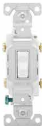
ETCS220W Commercial grade toggle switch, #14-10AWG, 20A, Commercial, Flush, 120/277V
