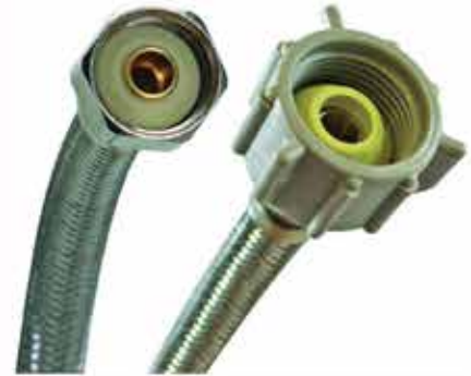
FMB1T20 3/8" Compression x 7/8" Ballcock x 20" Braided Stainless Steel Toilet Connector
